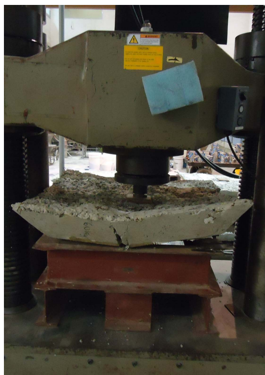
Fig. 2. Square panel test according to EN 14488-5.
