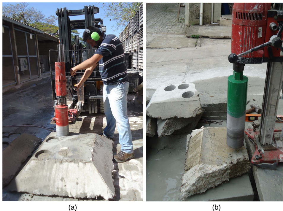
Fig. 3. Cylinder extraction from (a) large panels; and (b) small panels.
